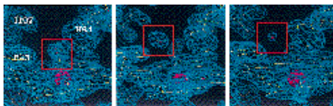
FIG. 5. Crystal structures of wild-type MbCO (left), photodissociated Mb*CO (middle), and deoxy-Mb (right) at 20 K in the P6 form. The electron density maps ( 2F_o - F_c ) were taken from Schlichting et al. (1994). The iron density is shown in red. The red square encloses, from left to right, bound CO, photodissociated CO, and non-coordinated distal pocket water. The iron atom is, from left to right, in the plane of the pyrrole nitrogens, partially out-of-plane, and completely out-of-plane, respectively (see Fig. 1).
